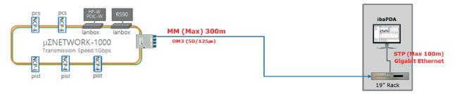
Case 2: When used at a distance of 300m to 2km (Gigabit Ethernet)
